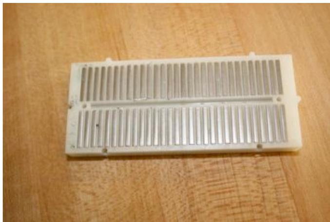
Each strip of metal is one node, or connection point, where parts can be connected together. Each node has five contacts or holes where circuit elements can connect to the node.
